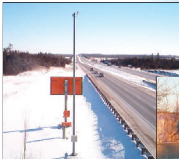
Left: A monitoring camera records traffic flow at the Salmon River test site. Bottom: A PVMS at Wymans Road, Salmon River, positioned in advance of the construction site.
